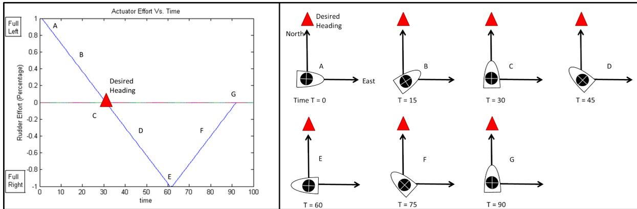
Figure 10: **Actuator Effort.** As the heading of the vessel deviates by a maximum degree (90 degrees), the actuator effort saturates in the respective direction. The effort starts to decrease as the vessel’s heading tends towards the desired. If it surpasses the desired heading to the other hemisphere, the rudder actuates in the opposite direction to correct for error.
