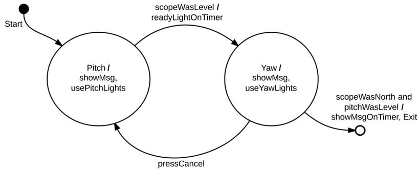
\* The user must hold the pitch level for 3 seconds while the two top lights are on to progress through each state.
