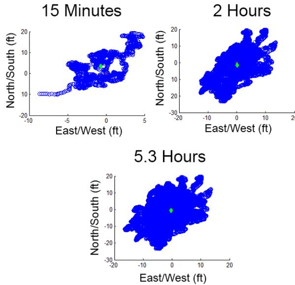
Figure 6: **GPS Error Convergence Test.** Measured error convergence in position of two GPS receivers over time.
