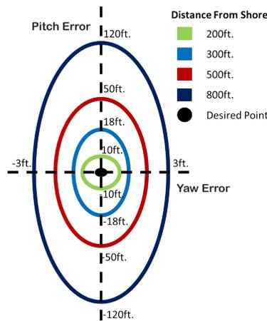
Figure 7: **Encoder Error from Resolution.** Uncertainty in measured position due to encoder resolution at various distances from the shore.
