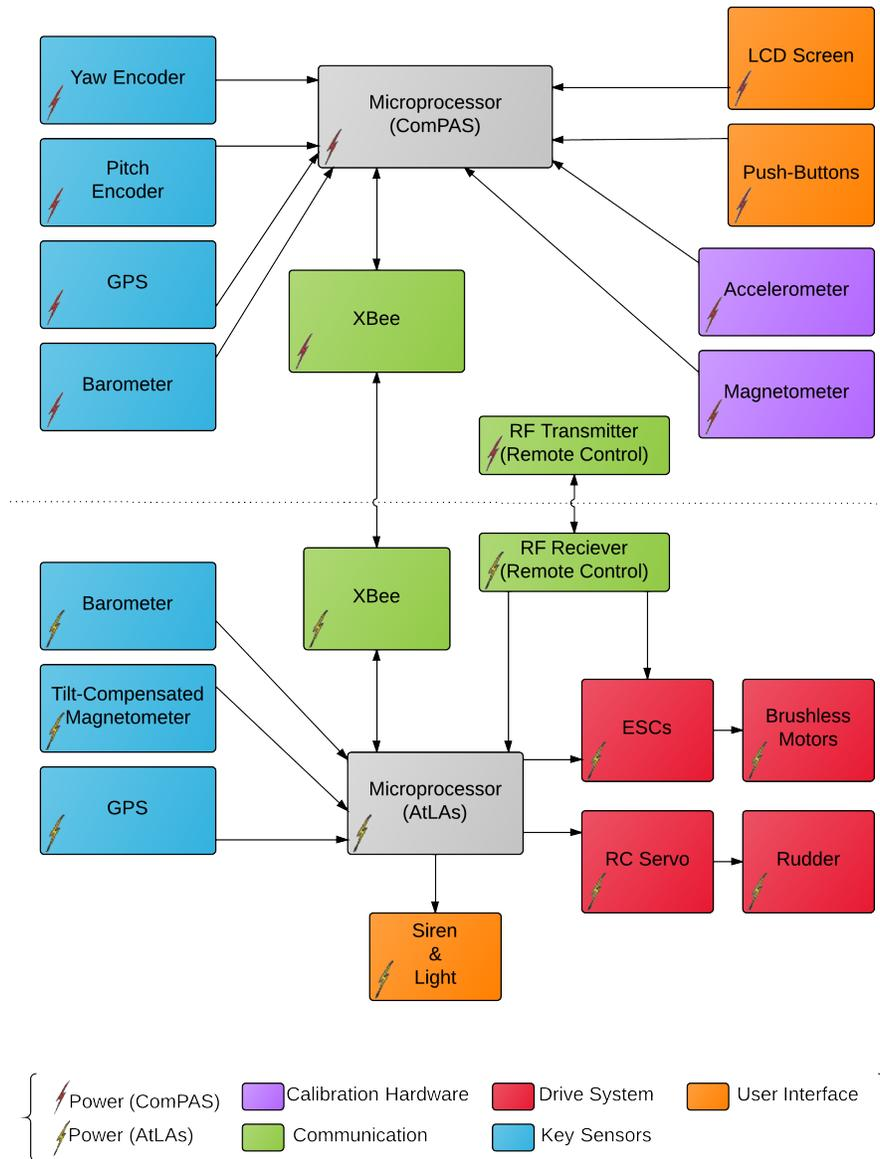
Figure 3: **Top Level Block Diagram.** Both sub-systems have their own respective sensor ensemble, user interface, and actuators. The common node is the communications which tie both systems together.
