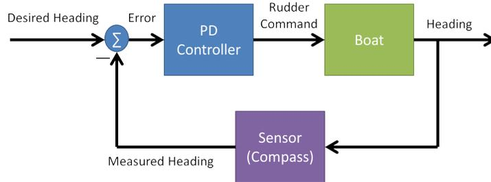
Figure 8: **AtLAs Feedback Control System.** The proportional-derivative control system for the AtLAs was implemented digitally using a microcontroller, and tracks a desired course heading towards the drowning person.
