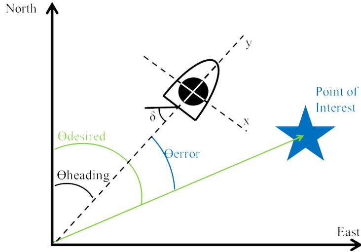
Figure 9: **Reference Frame.** The correction in heading is computed from the difference between the current heading of the vessel and the desired heading of the point of interest. The reference frame is with respect to the ComPAS as the origin.
