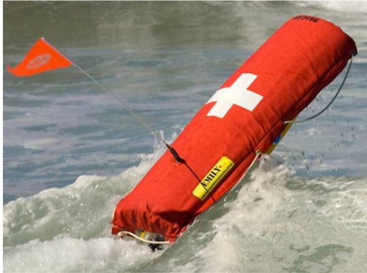
Figure 2: **E.M.I.L.Y (Emergency Integrated Lifesaving Lanyard)**. A remote controlled buoy designed by Hydronalix.
