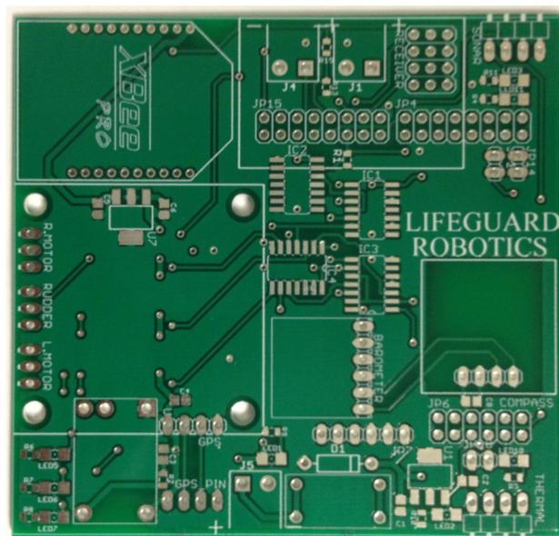
Figure 11: **AtLAs IO shield.** A custom printed circuit board for the AtLAs that serves as a shield for the microcontroller.
