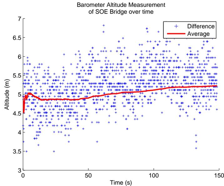
Figure 4: **Barometer Height Difference Test.** Time plot of the measured height difference between two barometers after low-pass filtering (red).
