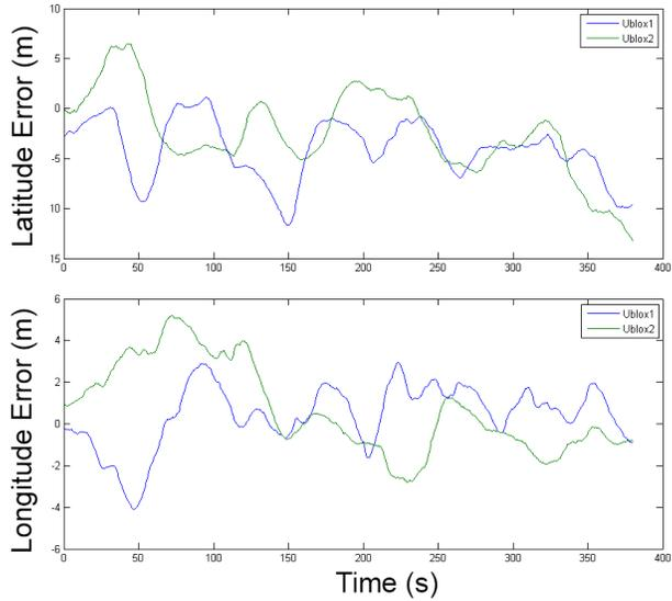
Figure 5: **GPS Error Correlation Test.** Correlation between the measured error of two GPS receivers in close proximity.
